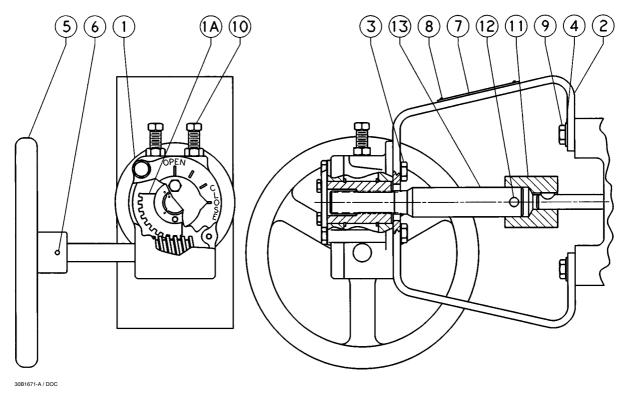
Figure 7. Type 1077 Actuator Assembly for Coupled or Keyed Shafts
